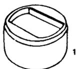
1. Flush-fitting pot socket for twist-locks and locator cones; sometimes referred to as a deck insert socket.
