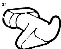
31. Penguin-hook for connecting lashing gear to container corner casting. Variations on this shape produce rhino-hooks, pad-hooks, viking-hooks, etc. It is important that the correct shape hook be used at the position for which it was designed.
